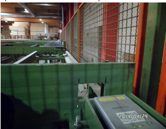
Fig 1: Dimetix Laser measures the wood face-on
