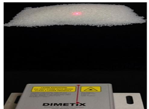
Fig 2: Dimetix Laser Sensor measures on white plastic pellets
