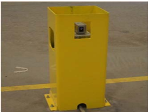
Fig 2: Built-in Dimetix Laser Sensor
