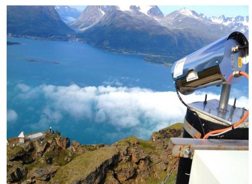
Fig 2: Laser measuring distance on reflector plate
