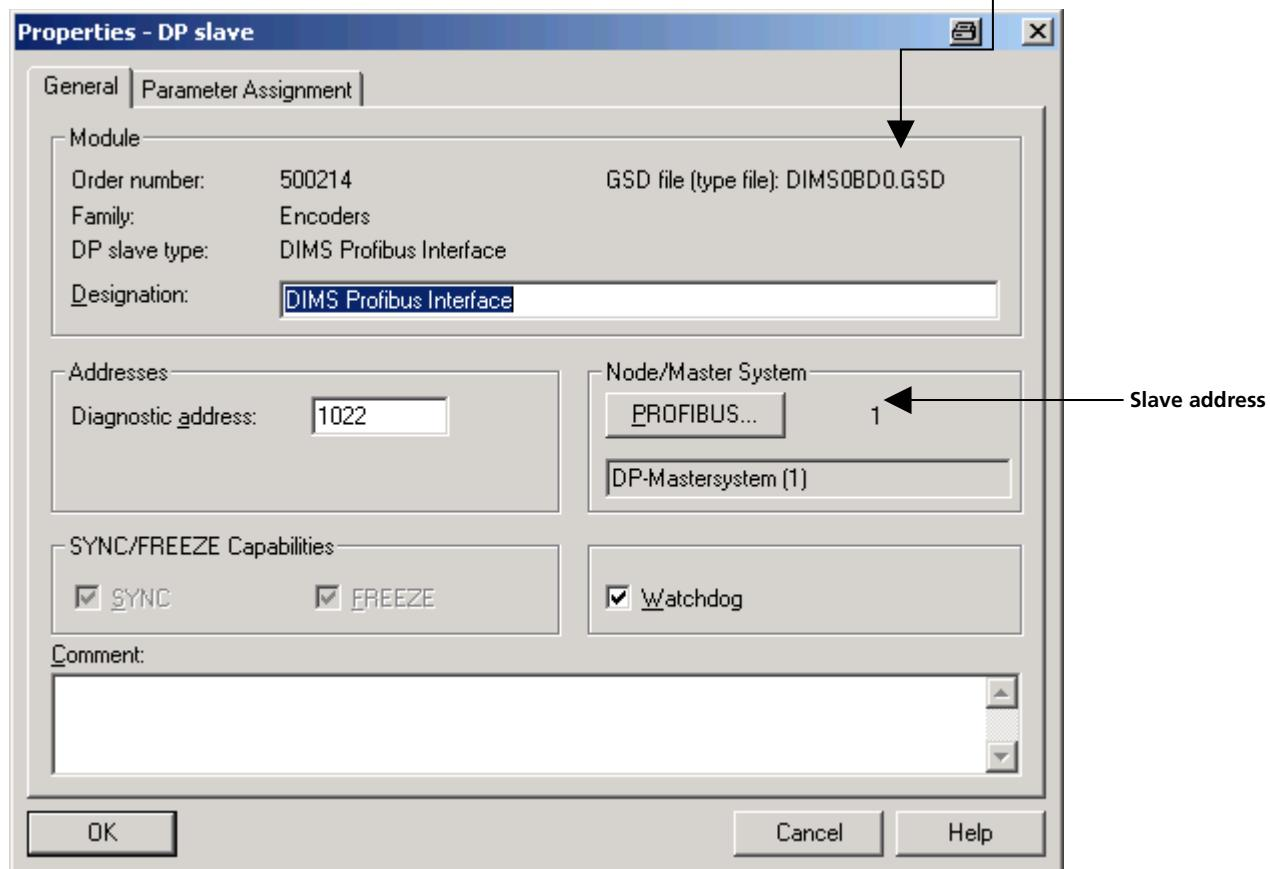
After the projection of the DIMS Profibus Interface, upload the appropriate module.
