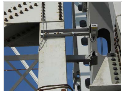
Pic 2: Mounted Sensor
