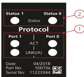
Identification of the existing status LED's of the exchangeable cover with Industrial Ethernet:
