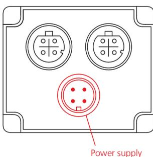
Figure 4: Connection diagram of the sensor power supply
