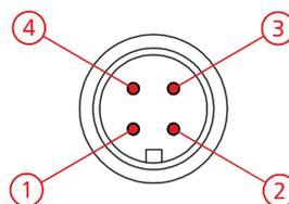
Connection diagram of power supply connector (M12 socket male, 4 pin, A coded):
