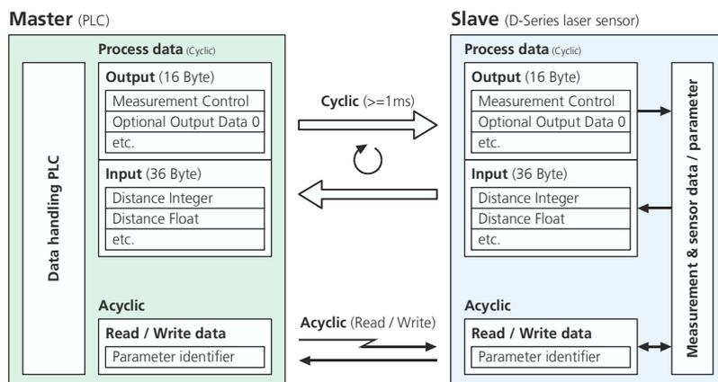
Figure 9: Cyclic (Process data) and acyclic communication between Industrial Ethernet Master (PLC) and the D-Series device with Industrial Ethernet interface.
