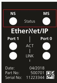
Figure 11: EtherNet/IP™ status LED's
